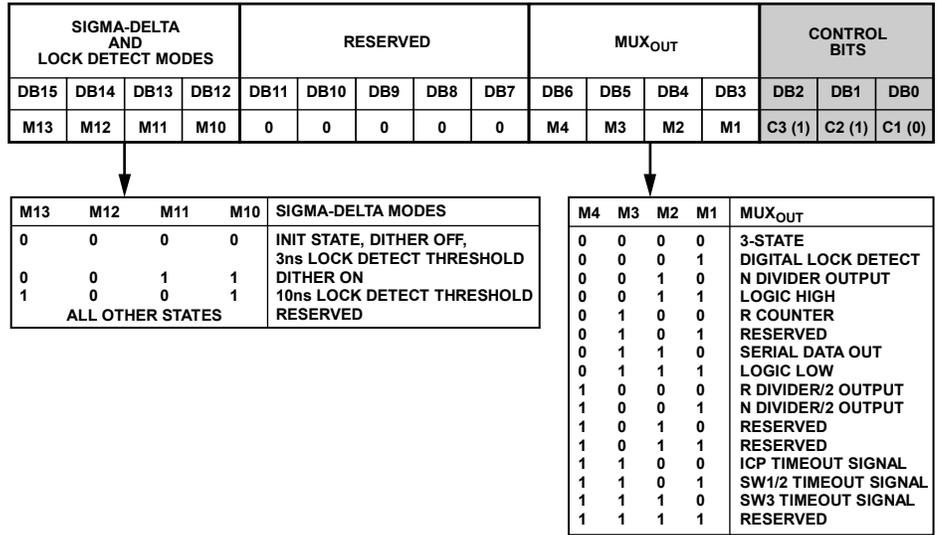
Figure 35. MUX Register (R6)
