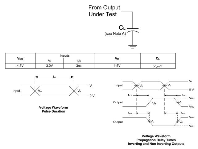
Notes: A. Includes test lead and test apparatus capacitance.
