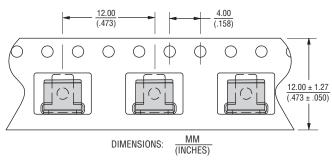
Unless otherwise specified, tolerances in decimals are .X  $\pm$  0.3, .XX  $\pm$  0.15 for lengths in millimeters and  $\pm$ 1 ° for degrees.
