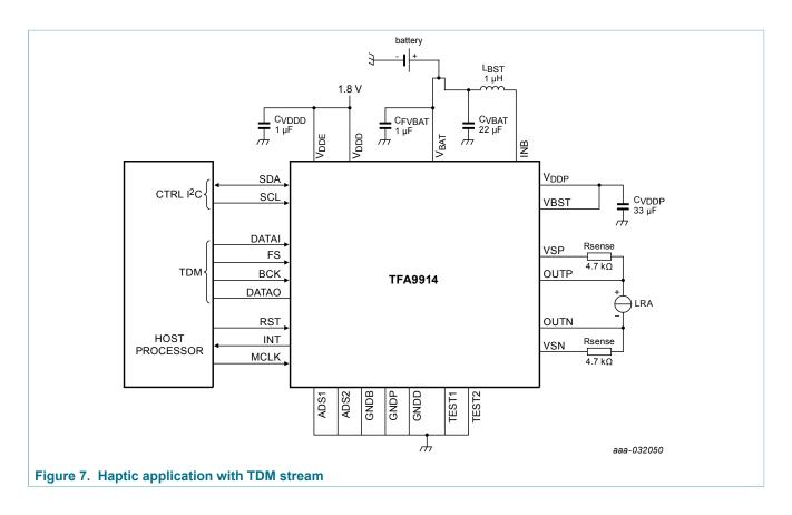
**High Efficiency Class-D Amplifier for Haptic**
