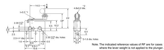
\*1. Stainless-steel lever \*2. Polyacetal resin roller
