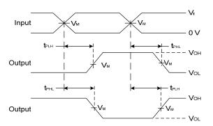
Voltage Waveform Propagation Delay Times
