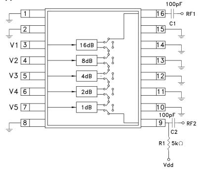
DC blocking capacitors C1 & C2 are required on RF1 & RF2. Choose C1 = C2 =  $100 \sim 300 \text{ pF}$  to allow lowest customer specific frequency to pass with minimal loss. R1 = 5K Ohm is required to supply voltage to the circuit through either PIN 9 or PIN 16.
