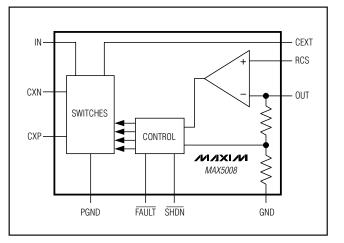
low-impedance trace, and connect the ground for  $C_{\rm IN},$   $C_{\rm EXT},$  and  $C_{\rm OUT}$  directly to PGND in a star configuration. Connect  $R_{CS}$  to  $C_{\rm EXT}$  through a short and low impedance trace.
