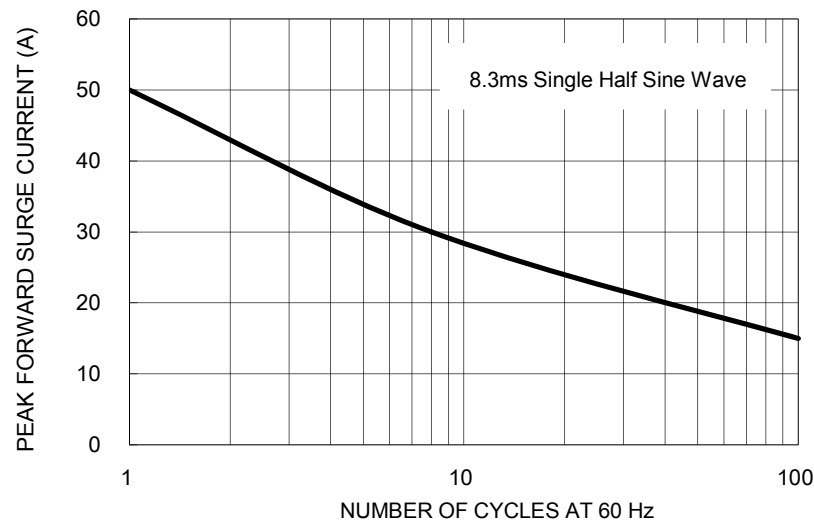
FIG. 3 MAXIMUM NON-REPETITIVE PEAK FORWARD SURGE CURRENT
