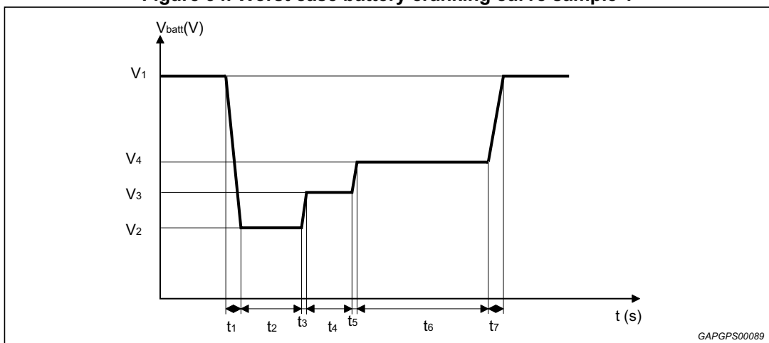
Figure 34. Worst case battery cranking curve sample 1
