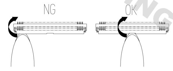
5. Do not lift or snag the actuator as shown in the figures below. This can result in damage. (Operate the lever only in a rotating fashion as instructed in paragraph 2 above.)
