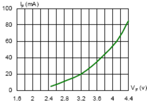
Fig.1 Forward Current vs. Forward Voltage
