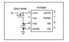
This method limits the +V<sub>IN</sub> voltage to  $V_{DD}$  +  $V_{GS(OFF)}$  of the depletion MOSFET for all input voltages and in fact raises the maximum allowable peak input voltage to the breakdown voltage rating of the depletion MOSFET. The worst-case power dissipation in the HV9906 is now given by the equation
