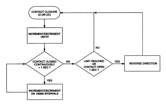
CONTACT OPEN AND CONTACT CLOSURE TIMING IS 1 SECOND  $\pm$  15%
