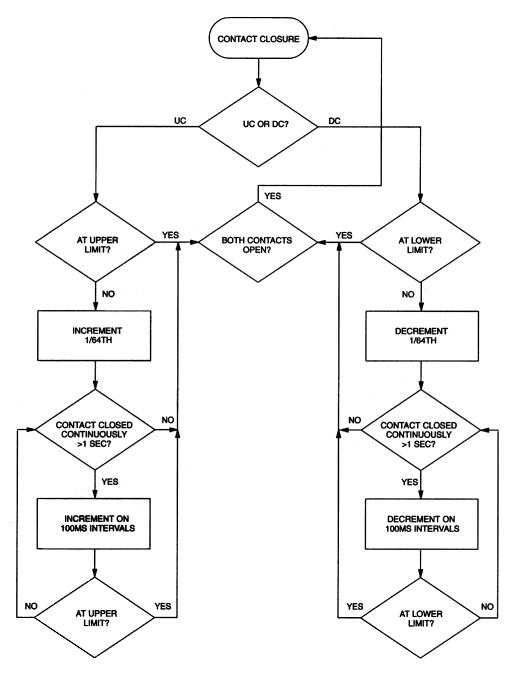
CONTACT OPEN AND CONTACT CLOSURE TIMING IS 1 SECOND  $\pm$  15%
