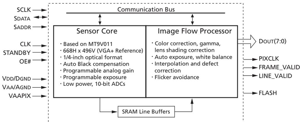
The MT9V111 can accept the input clock of up to 27 MHz, delivering 30 fps. With power-on defaults (see Appendix B for recommended defaults), the camera is configured to deliver 15 fps at 12 MHz and automatically slows down the frame rate in low-light conditions to achieve longer exposures and better image quality.
