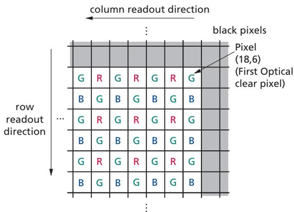
The sensor core image data is read-out in a progressive scan. Valid image data is surrounded by horizontal and vertical blanking, as shown in Figure 9. The amount of horizontal and vertical blanking is programmable through the sensor core registers Reg0x05 and Reg0x06, respectively. LINE\_VALID is HIGH during the shaded region of the figure. See “Appendix A – Sensor Timing” on page 20 for the description of FRAME\_VALID timing.
