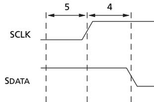
**Figure 21: Serial Host Interface Stop Condition Timing**
