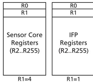
Note: Program R1 to select the desired space (4 = sensor core registers, 1 = IFP/SOC registers).
