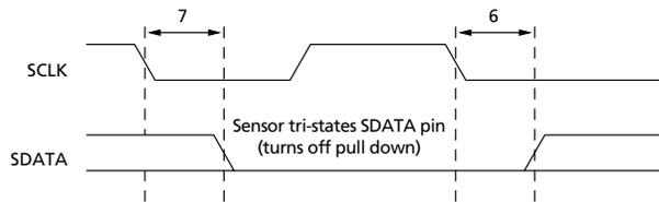
**Note:** After a read, the master receiver must pull down SDATA to acknowledge receipt of data bits. When read sequence is complete, the master must generate a no acknowledge by leaving SDATA to float HIGH. On the following cycle, a start or stop bit may be used.
