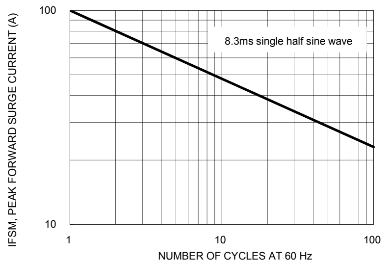
FIG. 4 MAXIMUM NON-REPETITIVE FORWARD SURGE CURRENT UNIDIRECTIONAL ONLY
