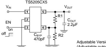
Adjustable Version:  $V_{OUT} = 1.24 (1+R2/R1)$  (Adjustable output range up to 8V)
