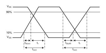
Switching time waveforms
