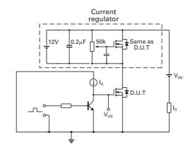
Gate charge test circuit
