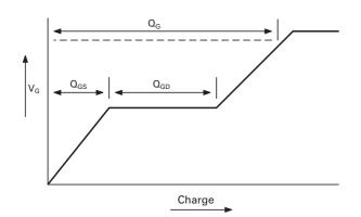
Basic gate charge waveform
