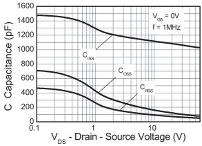
Capacitance v Drain-Source Voltage
