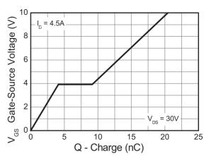
**Gate-Source Voltage v Gate Charge**
