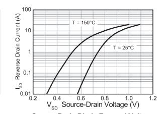
Source-Drain Diode Forward Voltage
