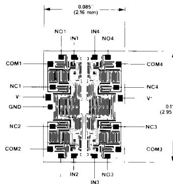
NOTE: NCx IS CONNECTED TO COMx WHEN INx IS LOW.
