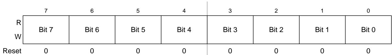
Figure 7-18. Debug Comparator A Register Low (DBGCAL)
