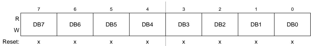
Figure 10-33. Data Segment Registers (DSR0–DSR7) — Extended Identifier Mapping
