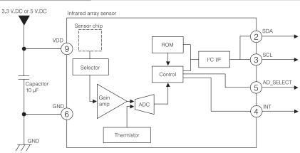
\* INT terminal ④ normally has same voltage as VDD. When interrupting, same as GND (0V)
