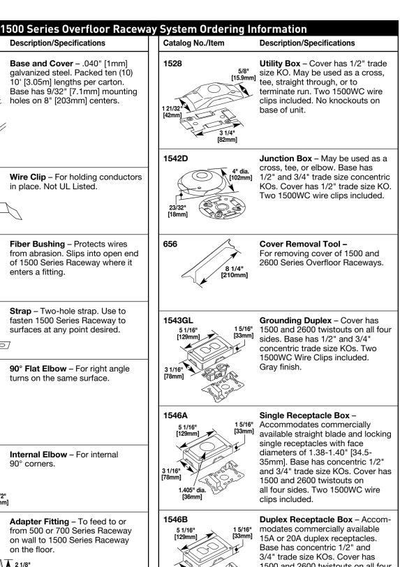
1500 and 2600 twistouts on all four sides. Two 1500WC wire clips included. Side wiring recommended.
