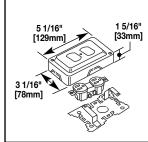
**Grounding Duplex** – Cover has 1500 and 2600 twistouts on all four sides. Base has concentric 1/2" and 3/4" KOs. Two 1500WC Wire Clips included.
