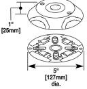
Junction Box - May be used with 1500 and/or 2600 as a cross, tee. or elbow. Cover has 1/2" trade size KO. Base has concentric 1/2" and 3/4" trade size KO to enable connection to floor, outlet boxes, or under floor duct systems (use chase nipple - not included). Two 2600WC wire clips included.
