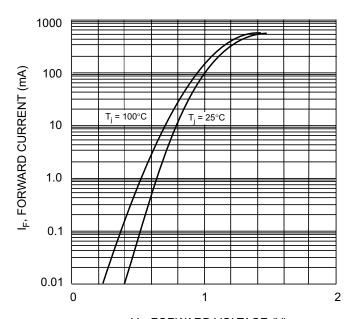
V<sub>F</sub>, FORWARD VOLTAGE (V) Fig. 2 Forward Characteristics
