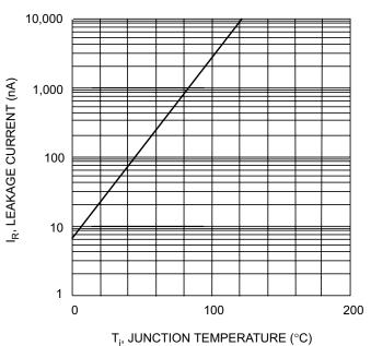
Fig. 4 Leakage Current vs Junction Temperature
