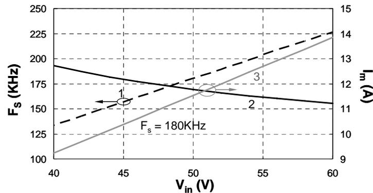
Fig. 3. Magnetizing current with constant and variable frequency.
