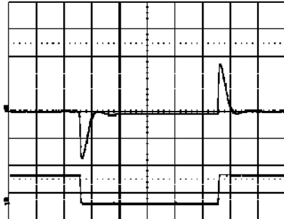
Output voltage response to load current step-change (5-15-5 A) at: T_{ref} = +25^\circ\text{C} , V_i = 53\text{ V} . Top trace: output voltage (100mV/div). Time scale: 0.1 ms/div.
