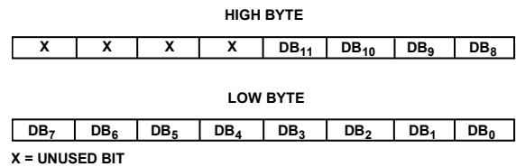
Figure 38. Data Format for AD5341
