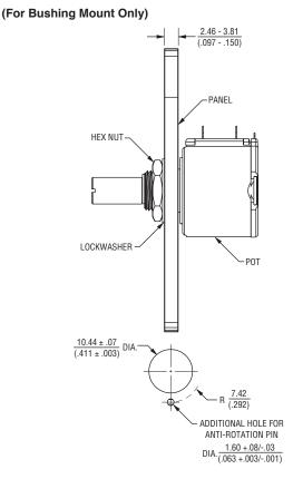
Anti-rotation pin hole is shown at six o'clock position for reference only. The actual location is determined by the customer's application. Refer to the front view of the potentiometer to see the location of the optional A/R pin.
