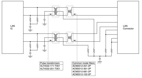
Note) Peripheral circuits differ depending on the IC used; check the circuits with the application note of the IC, etc.
