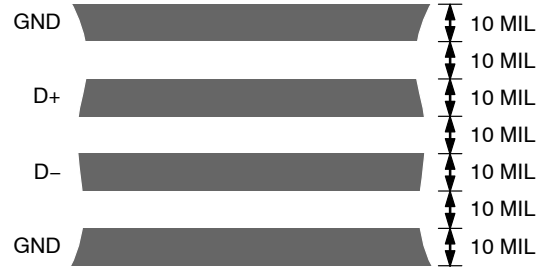
Figure 18. Arrangement of Signal Tracks
