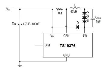
A value of 1uF will reduce the supply ripple current by a factor three (approx.). Proportionally lower ripple can be achieved with higher capacitor values. Note that the capacitor will not affect operating frequency or efficiency, but it will increase start-up delay and reduce the frequency of dimming, by reducing the rate of rise of LED voltage. By adding this capacitor the current waveform through the LED(s) changes from a triangular ramp to a more
