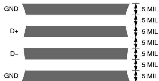
Figure 16. Arrangement of Signal Tracks
