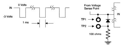
NOTE: This series of pulses must be applied during normal +5 volt operation.
