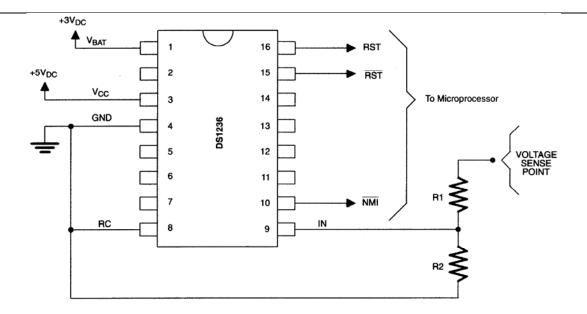
EXAMPLE 1: 5 VOLT SUPPLY, R2 = 10k OHM,  $V_{SENSE} = 4.80$  VOLTS
