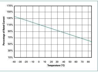
Note: Typical Temperature rerating curve, refer to table for derating data
