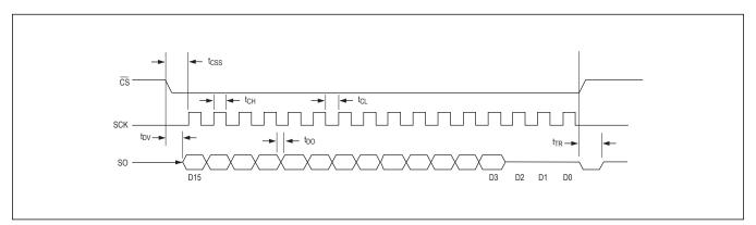
Figure 1b. Serial Interface Timing
