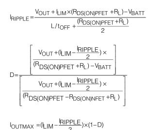
Here,  $I_{LIM}$  is the NFET current limit (800mA typ), tOFF is the LX switch's off-time (0.25µs typ), and  $R_L$  is the series resistance of the inductor.
