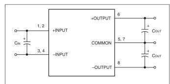
Figure 2. Using External Capacitors to Reduce Input/Output Ripple/Noise
