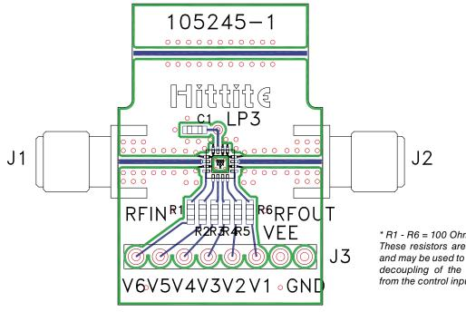
\* R1 - R6 = 100 Ohm. These resistors are optional and may be used to enhance decoupling of the RF path from the control inputs.
