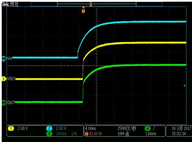
No-Load to Over-Load Transient Response ( V_{in}=5\text{V} , R_{load}=2.7\Omega )
