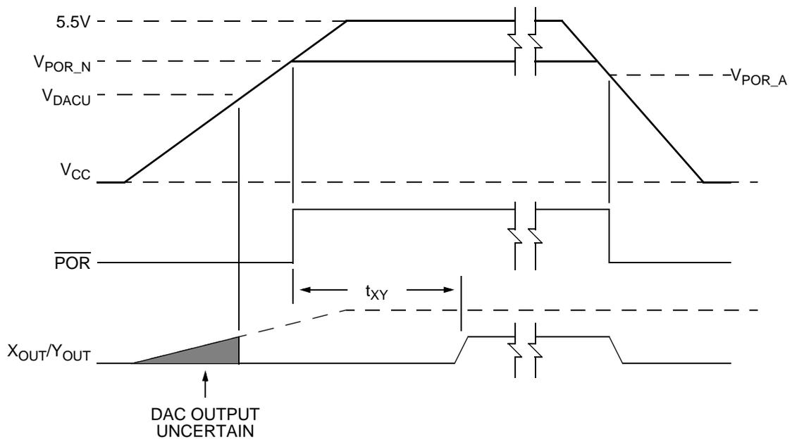
Figure 2-1 Power-Up Timing
