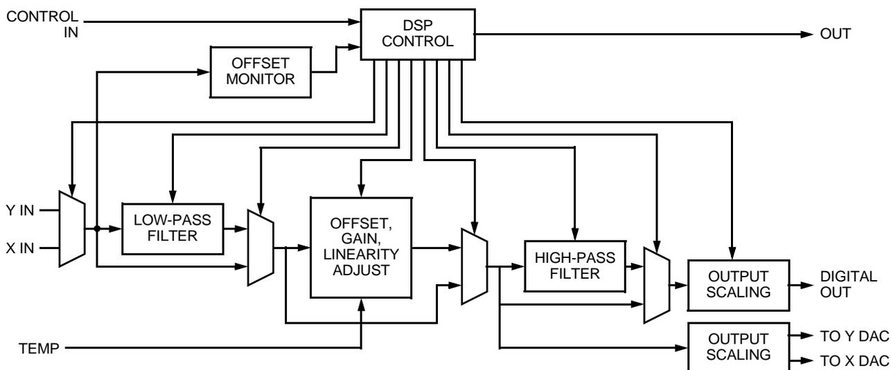
Figure 1-3 MMA62XXKEG DSP Block Diagram
