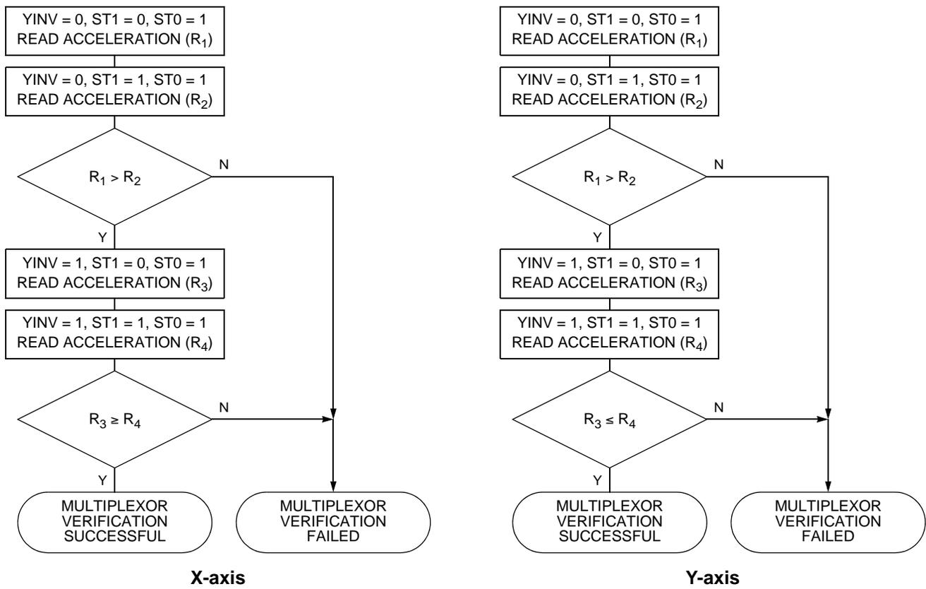
Figure 3-2 DSP Input Multiplexor Verification Flow Chart
