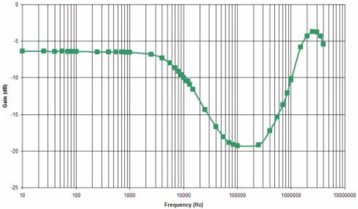
Figure 2-2 Power Supply Coupling - DAC Outputs
