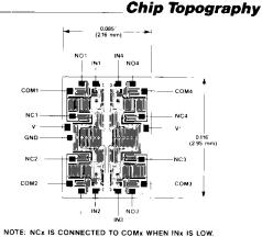
NOTE. NEX IS CONNECTED TO COMX WHEN INX IS LOW.
