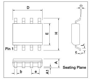
CONTROLLING DIMENSIONS ARE IN INCHES APPROX IN MILLIMETERS
